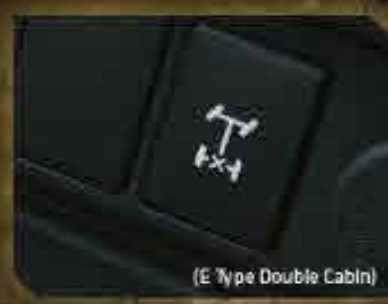
Rear Differential Lock System The system helps secure traction when driving in muddy terrain or in the unlikely situation when the vehicle is stuck (V, G, E Type Double Cabin; Single Cabin DSL 4x4)
