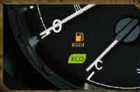
Eco Lamp Indicator The Eco Lamp Indicator helps you to get more miles out of each tank of gas and drive more efficiently (All Type)
